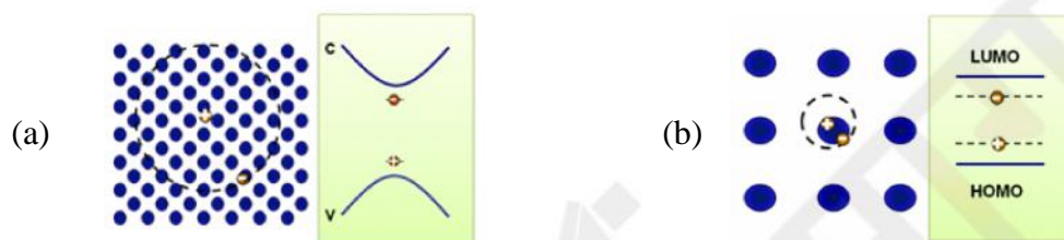
Figure 1. Shown the comparison relation between the Wannier-Mott and Frenkel excitons. (a) Wannier-Mott excitons and (b) Frenkel excitons.
